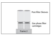
Frame 2 contains the four gas phase filter cartridges with the four post-filter sleeves. Remove frame 2 with the cartridges.
