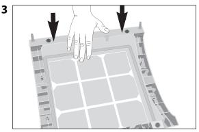
Press down until the mounting rail snaps into place. Repeat with second rail.
