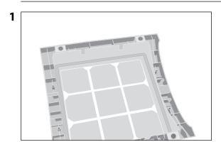
Turn the device upside down on a soft and clean surface.
