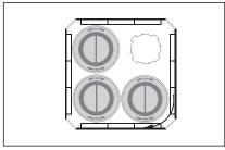
5. Insert the new cartridges in the base plate by turning the cartridge clockwise. Finally check that each cartridge is well secured in the base plate.
