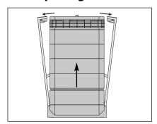
Open the locking arms, making sure they are fully extended outward. For details, refer to the section 6.3.
