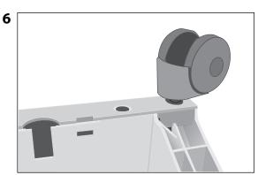
Ensure that each caster is securely fitted before placing the air purifier in its upright position onto the casters.
