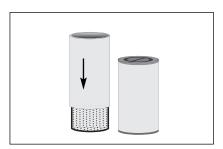
**4.** Pull a new filter sleeve over each new cartridge until it is completely covered.
