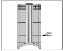
Opening the arms will cause the upper part of the housing to separate from frame 1. This will leave a narrow gap.
