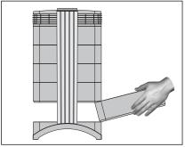
**3.** Place your hands on opposite sides of frame 1, lift it slightly and pull it out slowly. As the frame is withdrawn from the system, tilt it progressively upward to remove it completely.
