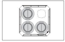
3. Twist each cartridge counter clockwise as far as it will go. It can then be lifted out of the base plate by hand.\*
