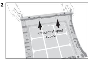
Place the mounting rail on the purifier's base so that the holes line up with the black connector pins on the base. The cut-ins should face the center of the unit.
