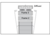
**1.** Open the locking arms, remove the diffuser and frame 3.
